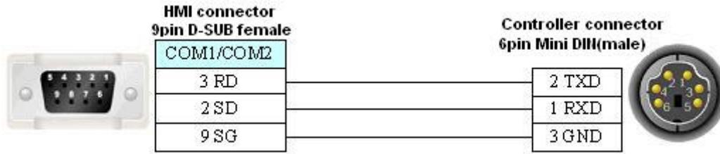
RS232 communication cable for C24 communication module
